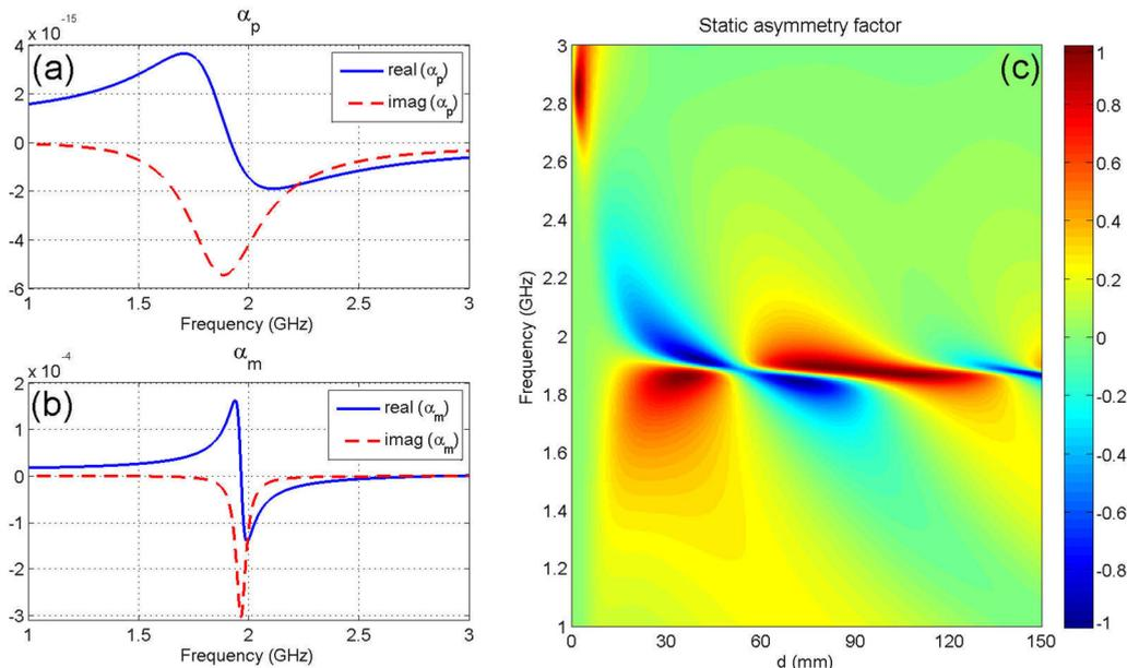
FIG. 3. Properties of the static configuration: (a) polarizability of the wire as a function of frequency, (b) polarizability of the split ring versus frequency, and (c) color map of the static asymmetry factor as a function of frequency (vertical axis) and separation distance between the wire and the ring (horizontal axis).
